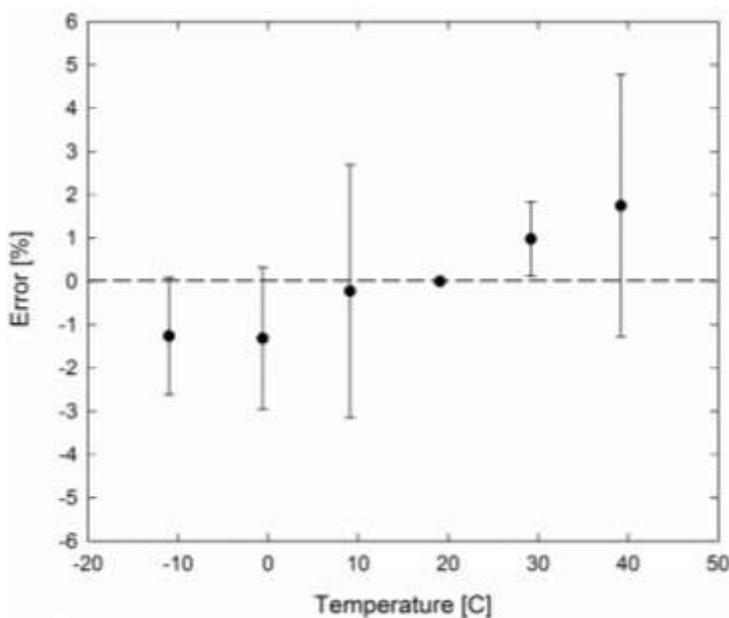
Mean temperature response of eight SQ series quantum sensors (**errors bars represent two standard deviations above and below mean**).
