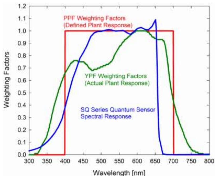
Radiation weighting factors for PPF (defined plant response to radiation), YPF (measured plant response to radiation), and Apogee SQ Series quantum sensors (sensor sensitivity to different wavelengths of radiation).
