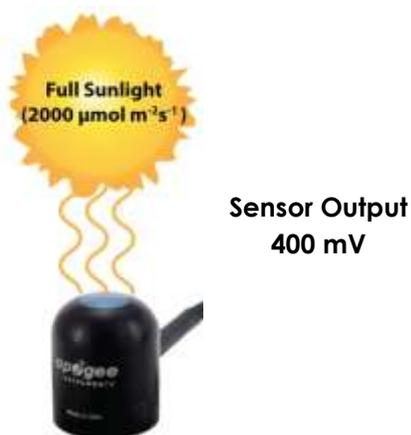
Example of PPF measurement with an Apogee quantum sensor. Full sunlight yields a PPF on a horizontal plane at the Earth's surface of approximately  $2000 \mu\text{mol m}^{-2} \text{s}^{-1}$ . This yields an output signal of 400 mV. The signal is converted to PPF by multiplying by the calibration factor of  $5.00 \mu\text{mol m}^{-2} \text{s}^{-1}$  per mV.
